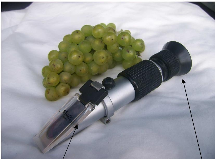
Squeeze the juice of one grape on the prism (under the Perspex lid) and close the lid down on to the juice, trying not to leave air bubbles. Hold up to the light and view through the eye piece
